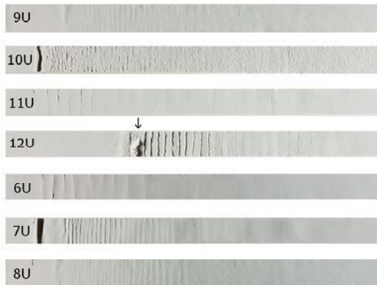
Figure 8: Severity of buckling caused by the test procedure.
