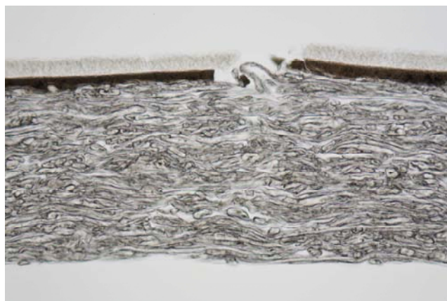
Figure 2: Cross-section photomicrograph of an inkjet paper showing buckling.
